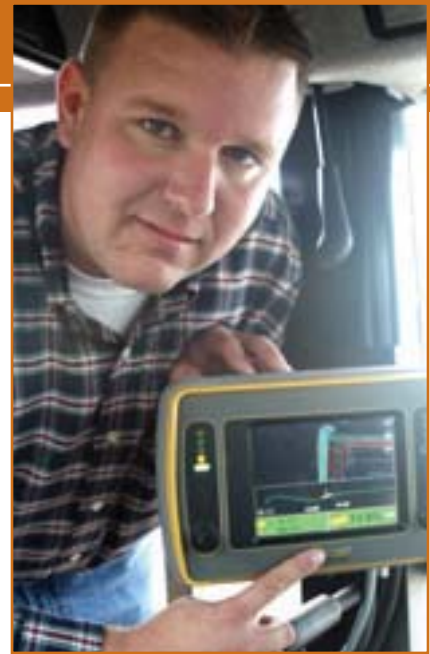
On the machines, the GPS system consists of a touch-screen monitor, a satellite receiver box and satellite antenna.
