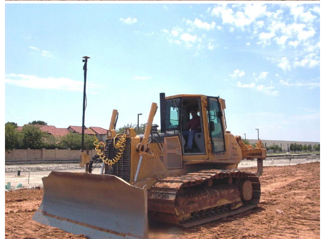
L & K's John Deere 850C with Topcon's System Five 3D-GPS+ automatic machine control
